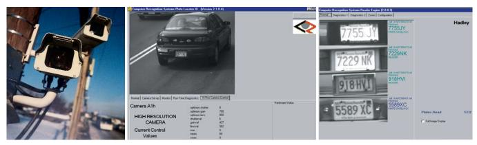
**Road tools.** Web-accessible video cameras installed near Northampton, MA, by the University of Massachusetts Transportation Center overlook the Calvin Coolidge Memorial Bridge on Route 9 (left). Two additional cameras photograph individual cars crossing the bridge (middle) and send the images to computers that isolate license plates and use machine vision algorithms to read the plate numbers (right). Once a plate has passed both cameras, the car's travel time is computed.
